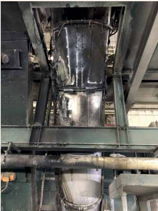
New vertical chute and high speed conveyor
