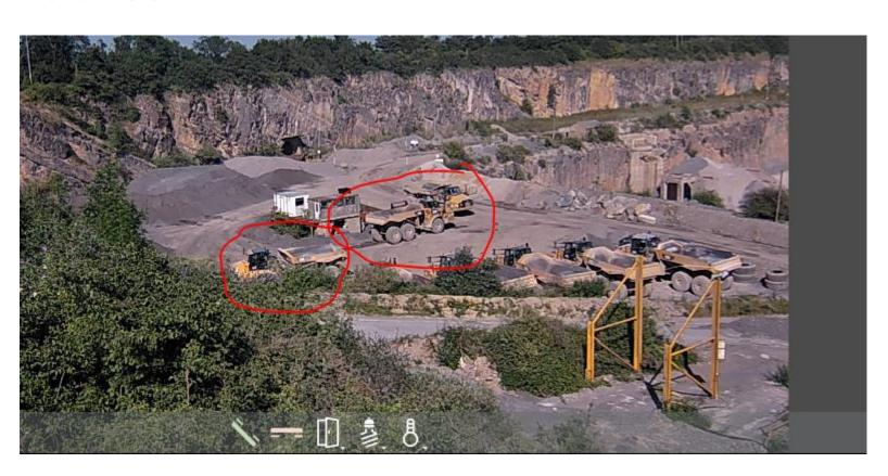
Previous problem.. A significant near hit when a shovel loading the 2/6mm pile reversed into a parked dumper.
