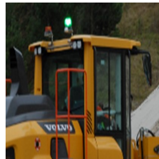
Green light on cab to indicate seatbelt is being worn
