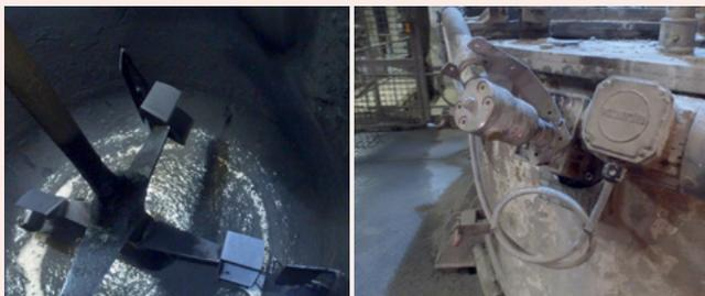
To mitigate these risks a new mixer wash system has been introduced. The mixer has been fitted with four rotating spray heads, each spray head delivers 50 litres of water every minute and operates at a pressure of 110bar. When activated one spray
