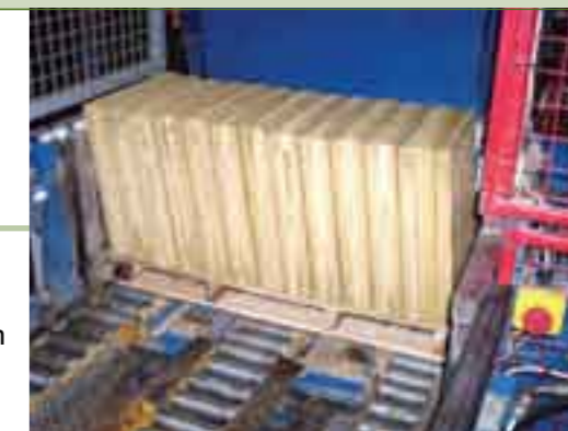
Slabs collated onto a pallet leaning against a support rail
