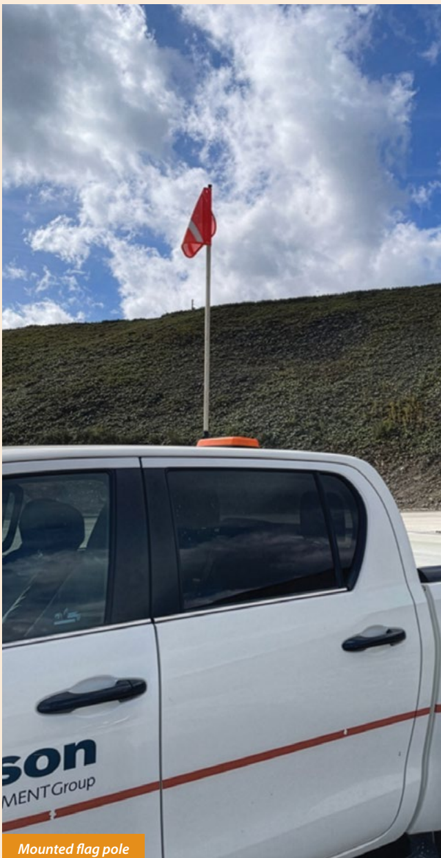
Fitting flag pole at ground level
