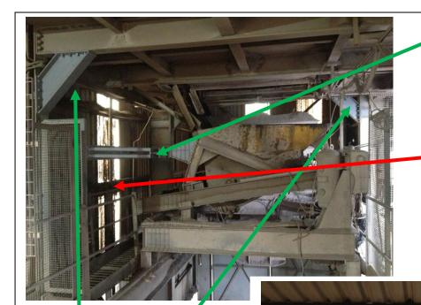
The Crumple Zone energy impact beam is attached to main structure to absorb the high energy impact without structurally weakening the integrity of the plant
