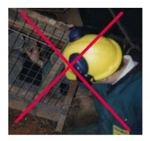
If you find defective or loose guards - **DON'T WALK BY** - if you can refit and secure the guards, then do so. If you can't, then make the site safe and report the defect to your Supervisor or Manager **IMMEDIATELY**.
