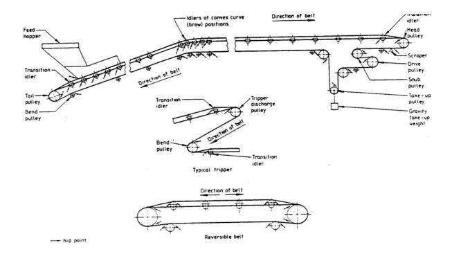
Entrapment between the moving conveyor and the rotating pulley or drum will always result in an injury that can often be fatal.
