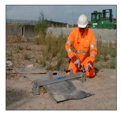
Where a knife has to be used to cut conveyor belting, always cut away from the body if possible.
