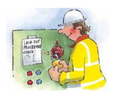
All isolation handles are fitted with a device that allows the handle to be locked in the contactor open (equipment isolated) position.
