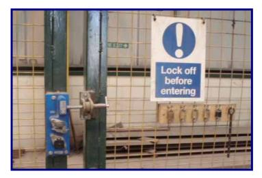
Whenever working on equipment (such as maintenance activities) protected by a Castell interlock, ALWAYS isolate and lock off the electrical supply with a personal padlock before starting work.
