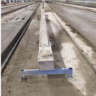
Spreader beam with stabiliser
