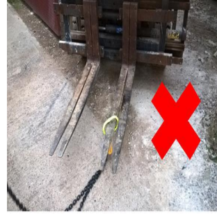
Lifting device used in incident
