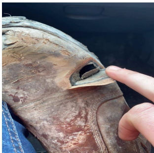
Damage to the boot above toe cap
