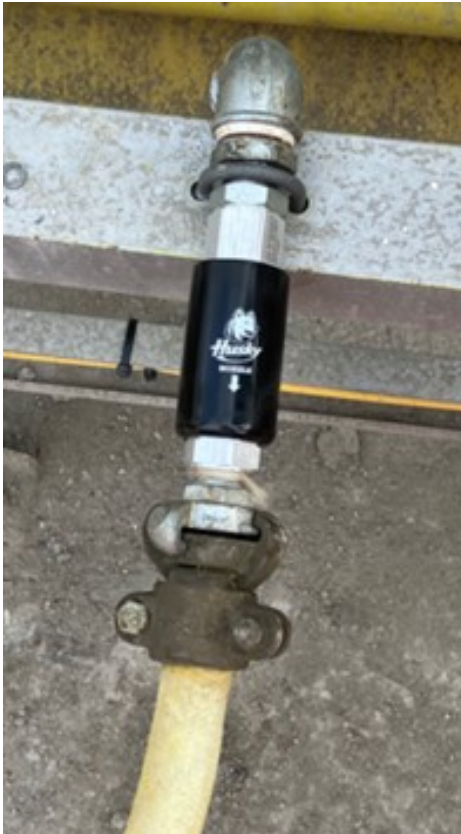
Image above shows a magnetic coupling in place and a typical example of a connection without one.
