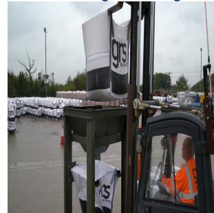
After - bagging frame
