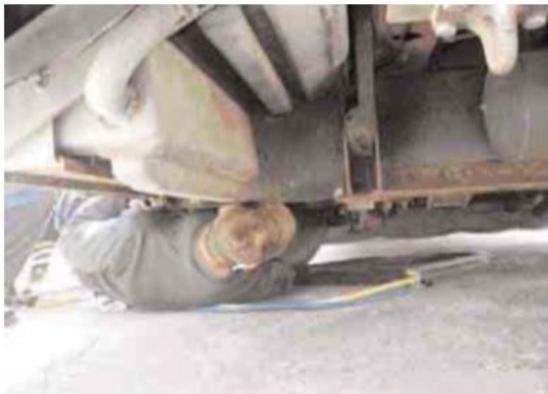
Vehicle ground clearance can suddenly and unexpectedly change due to a drop-in air pressure. This presents crushing and trapping hazards to technicians repairing vehicles, especially if working beneath them. There is also a risk of trapping around the wheel arch.
