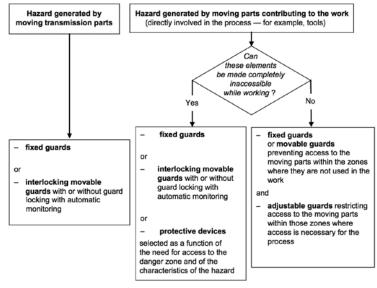
Figure 4 — Guidelines for choosing safeguards against hazards generated by moving parts
