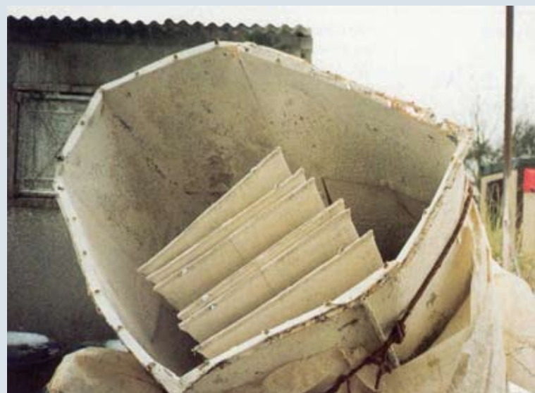
An over-pressurisation incident led to the 'launching' of this filter housing from the top of a silo. If this had landed on anyone, they would have been killed.
