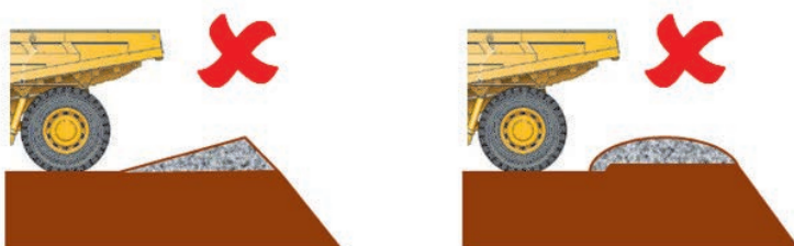
UNSUITABLE EDGE PROTECTION BERM PROFILE
