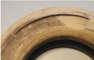
Figure 1 Zipper failure like this can lead to fatalities
