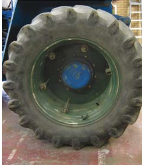
Figure 8 Divided wheel on a shovel loader
