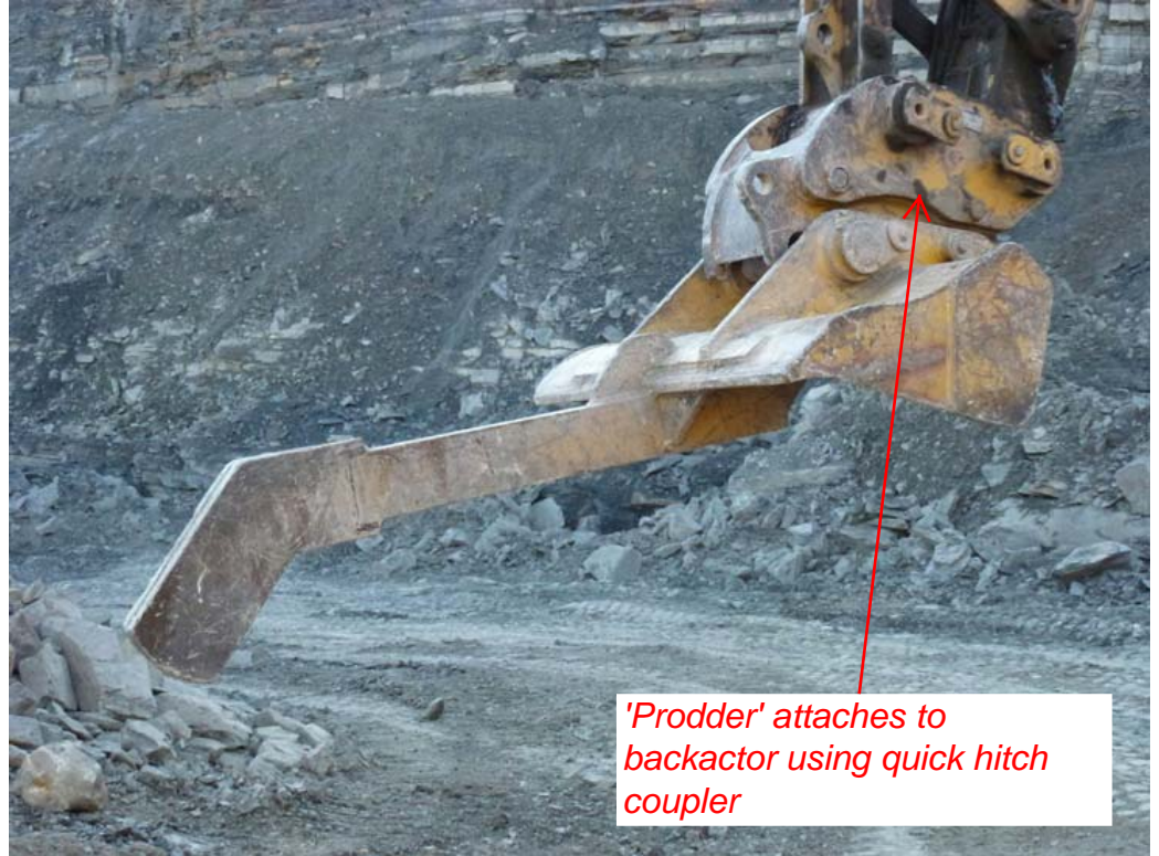
Backactor operator positions the 'prodder' above the rock between the wheels of the truck, the rock is removed in a downward motion so any stored energy is directed into the ground.
