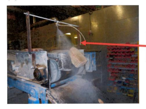
As blocks ejected from the waste conveyor, water used to suppress dust
