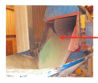
Exit from Rumbler drum open – extraction unit unable to draw dust away thus allowing to enter the atmosphere
