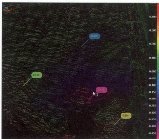
Fig. 14. Displacement measurements between successive rock face monitoring surveys showing expansion of the rock mass (green) and rockfall location (blue and pink)
