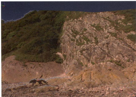
Fig. 1. Scan of a coastal rock face where each point has an ROB (red green blue) value allocated to it from the associated digital photograph (note: figure 1 is not the photograph but an actual screen shot from the 3D model)
