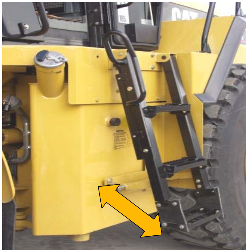
Inclined ladder actuated by parking brake with 15° slope for unmatched cab access and egress
