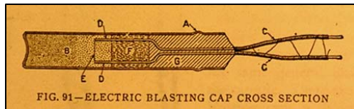
FIG. 91—ELECTRIC BLASTING CAP CROSS SECTION
