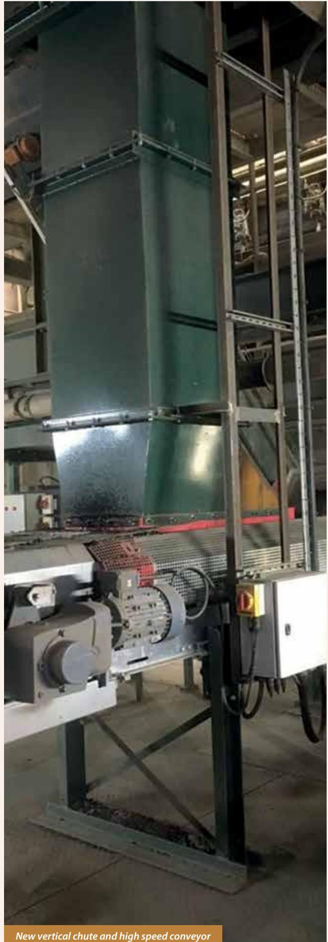
*New vertical chute and high speed conveyor*
