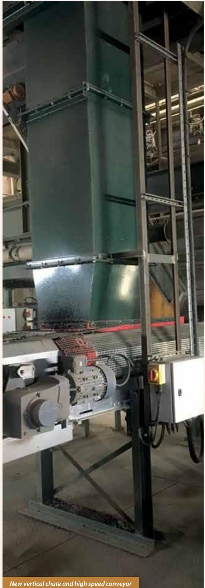
*New vertical chute and high speed conveyor*
