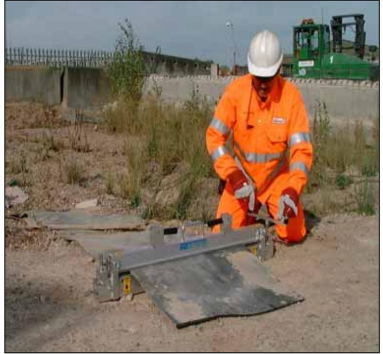
Where a knife has to be used to cut conveyor belting, always cut away from the body if possible.
